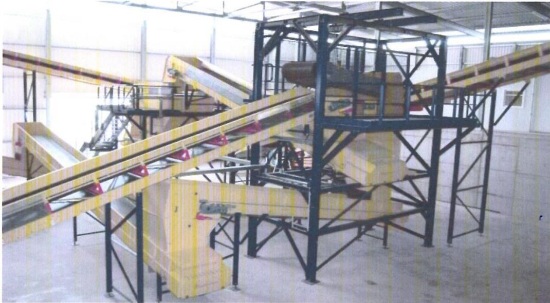
**Ferrous separator (Electro overband magnet)**
