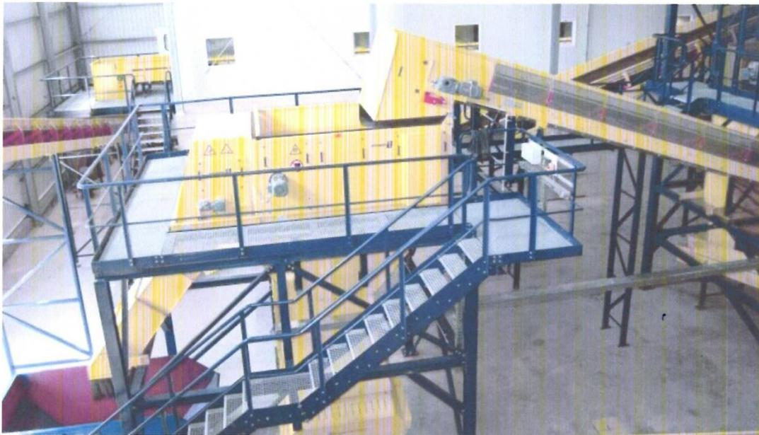
**Non-ferrous metals separator (Eddy current)**
